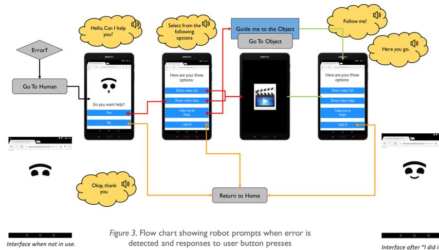
Figure 3. Flow chart showing robot prompts when error is detected and responses to user button presses
